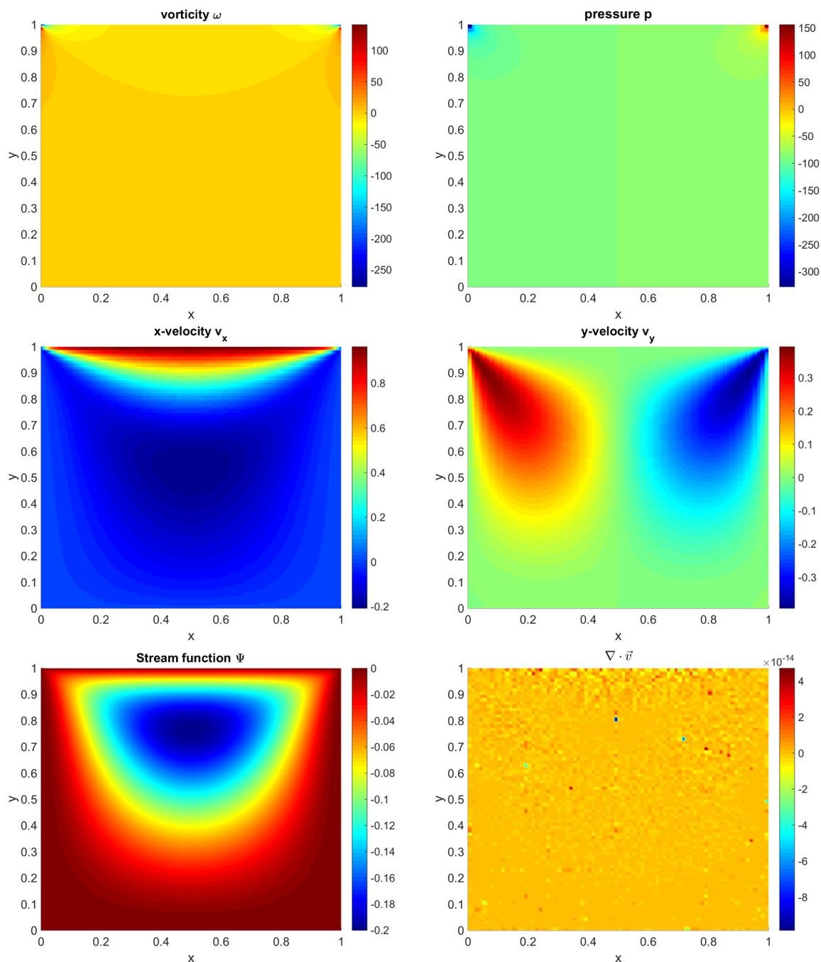
Figure 9: Lid-driven cavity flow solution on 80x80 grid
