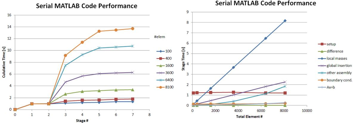
Figure 10: Time analysis of the serial MATLAB program
