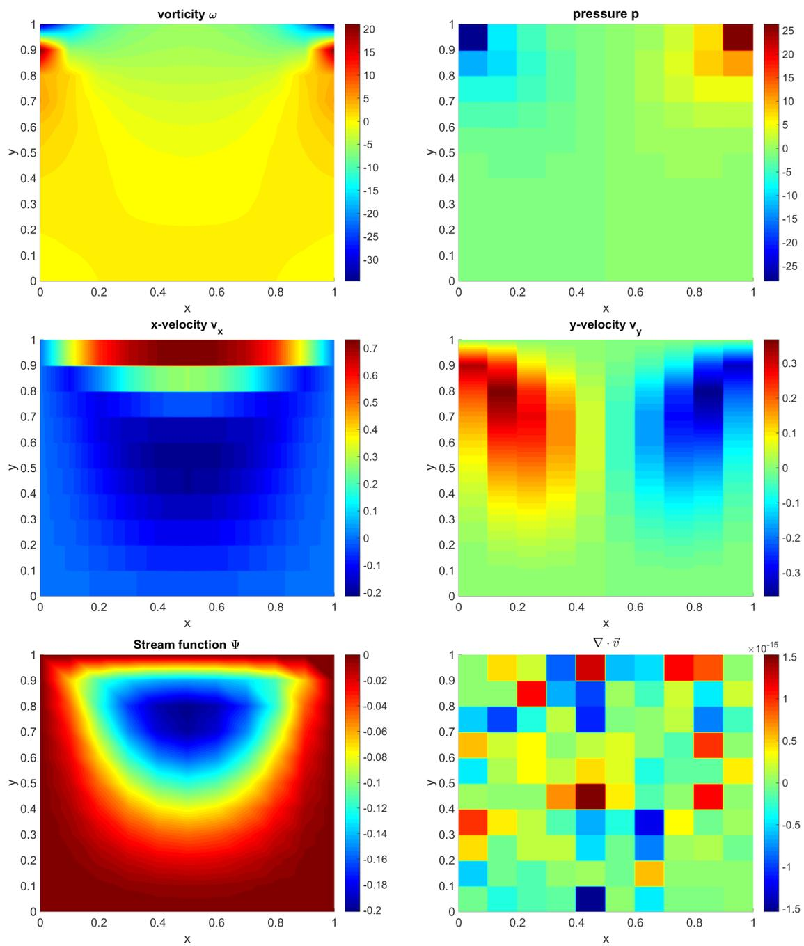
Figure 7: Lid-driven cavity flow solution on 10x10 grid
