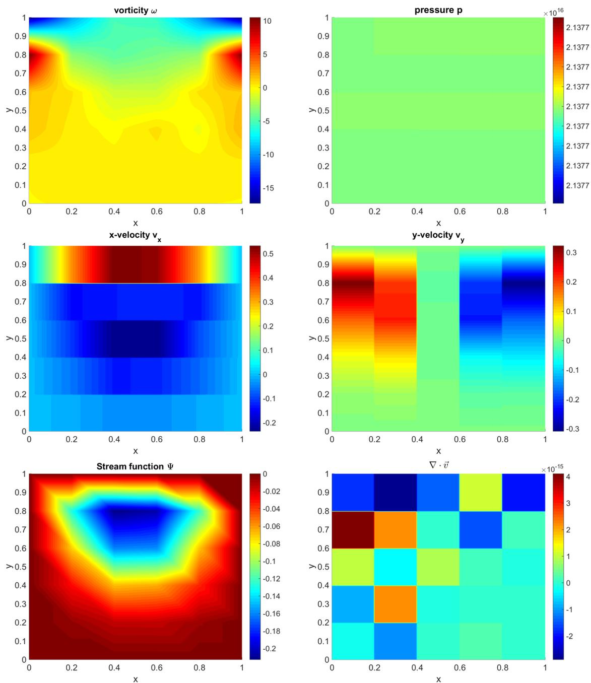
Figure 6: Lid-driven cavity flow solution on 5x5 grid
