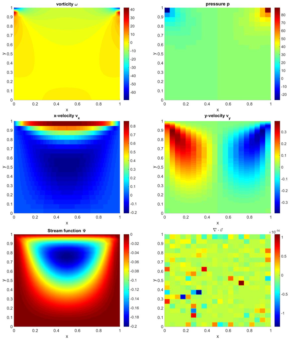
Figure 8: Lid-driven cavity flow solution on 20x20 grid
